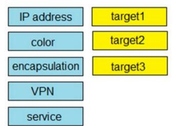
A TLOC, or Transport Location, is the attachment point where a WAN Edge router connects to the WAN transport network. A TLOC is uniquely identified and represented by a three-tuple, consisting of system IP address, link color, and encapsulation (Generic Routing Encapsulation [GRE] or IPsec).
