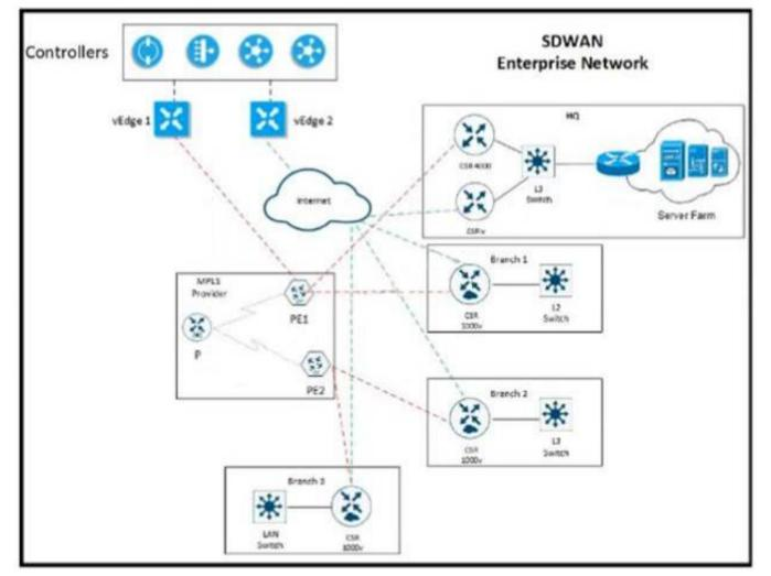
The network team must configure EI GRP peering at HQ with devices in the service VPN connected to WAN Edge CSRv. CSRv is currently configured with
